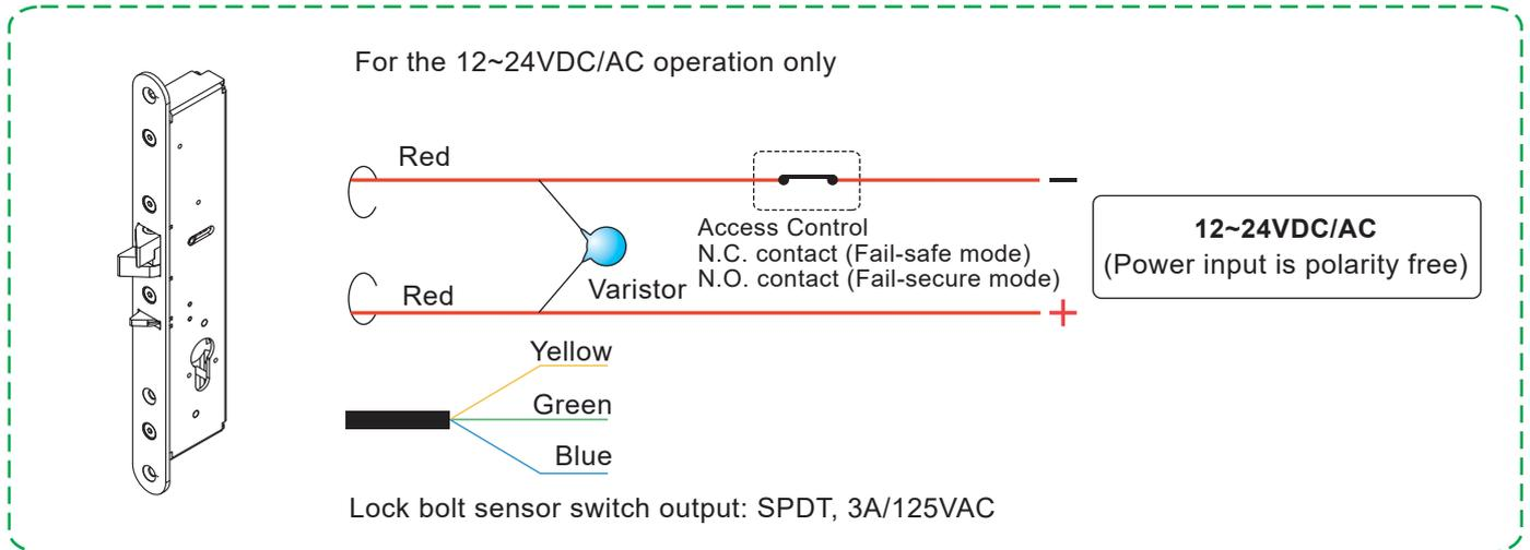
**NOTE:** The varistor (or diode) must be connected across the terminals as shown above. This protects the electromechanical lock from spikes and surges.
