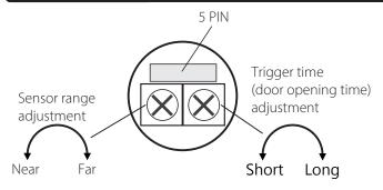
Note: Adjusting door opening time to maximum (turning all the way to the right) will set the switch to toggle mode.
