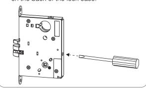
2. Push forward the flathead screwdriver, and the latchbolt will also be moved forward.
