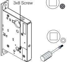
When the 3 x 8 screw is installed, turning the inside/outside lever retracts the latchbolt and opens the door. Lever rotation is monitored.
