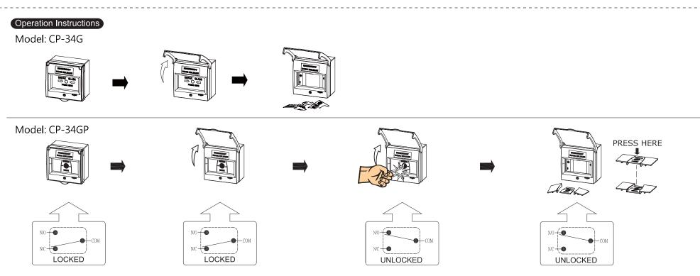
Open the clear plastic cover. Press harder to break the plastic glass so that the internal switches will change status from NC to NO, triggering the connected devices.
