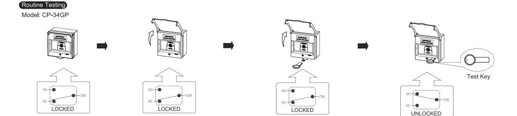
Open the clear plastic cover. Insert the test key into the hole so that the plastic glass will tilt to one side and the internal switches will then change status from NC to NO. Remove the test key so that the switches revert back to NC status.
