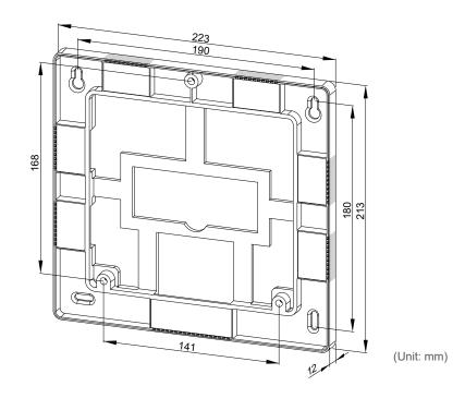
The mounting bracket is suitable for wall installations where wires are exposed. The mounting bracket makes installation and wiring quicker and easier and allows wires to be connected to the power supply from all sides.
