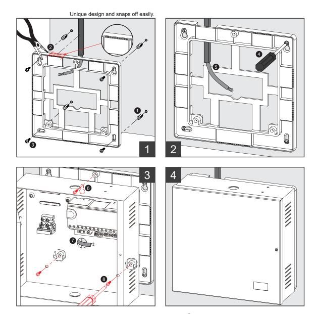
Figure 1 Drill holes on the wall as shown in 1 and rotate or adjust the mounting bracket according to the location of the power cable. 2 Snap off the removable parts of the board using pliers and pass the power cable through. 3 Install wall plugs and fix the mounting bracket with screws.
